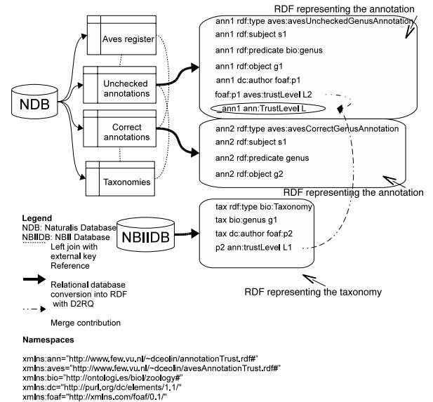
Figure 4: Case study overview. Given the two initial databases, we create RDF representations of annotations and taxonomies. Afterwards, we merge all reputations available in order to obtain a unique trust value for the annotation.
