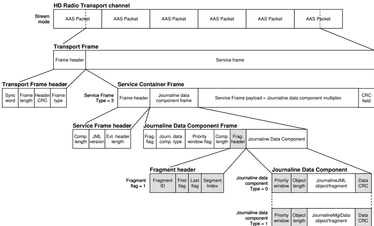
Figure 2: Protocol stack of Journaline adaptation layer over the HD Radio system.
