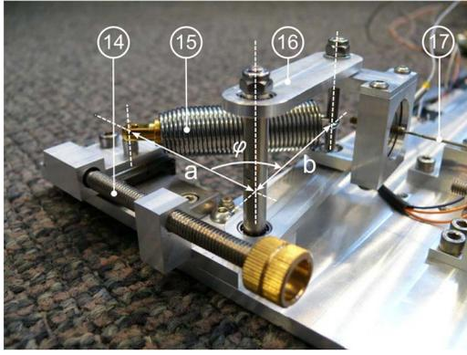
**Fig. 6** Constant force actuator, where (14) is the screw to adjust length  $a$ ; (15) is the nearly zero-free-length spring generating a force  $F_s$ ; (16) is the lever arm of length  $b=50$  mm and rotation angle  $\varphi$ ; and (17) is the actuation cable that applies a force  $F_a$  on the finger
