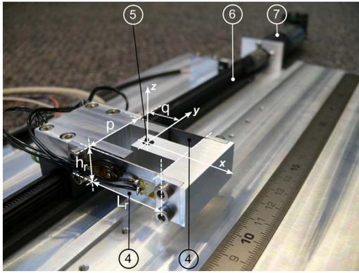
**Fig. 3** Load cell based on a straight line guidance with leaf springs, where (4) are leaf springs of thickness  $t$ , length  $L_r$ , and height  $h_r$ , mounted on a distance  $p$ , according Table 1; (5) is the hole in the slider where the shaft of the object is mounted on a distance  $q=L_r/2$  from the base; (6) is the lead screw; and (7) is the DC-motor
