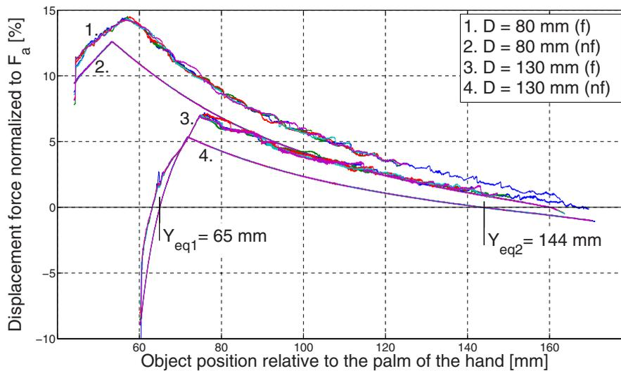
**Fig. 7** Measured forces to displace the object all the way out of the hand, where the repetitive measurements are shown on top of each other by different colors. The force is expressed as percentage of the actuation force of the finger.  $D$  denotes the object diameter, while ( $f$ ) and ( $nf$ ) denotes contact with and without friction, respectively. For experiment 4, the equilibrium positions  $Y_{eq1}$  (stable power grasp) and  $Y_{eq2}$  (unstable pinch grasp) are identified.
