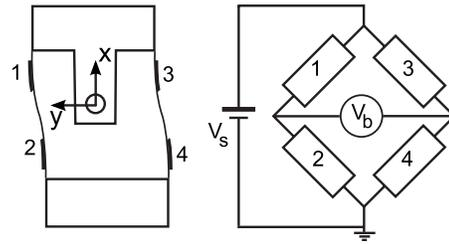
**Fig. 4** Schematic drawing of the top view of the load cell (left side) and Wheatstone's bridge configuration (right side) with the four strain gauges (1, 2, 3, and 4), supply voltage  $V_s$ , and voltage across the bridge  $V_b$
