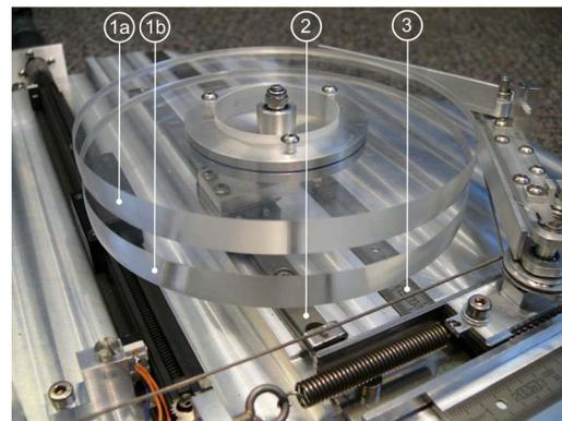
**Fig. 2 Picture of a freely moving object consisting of two independently rotating disks to assess frictionless grasping, where (1a) is the upper disk in contact with the distal phalanx; (1b) is the lower disk in contact with the proximal phalanx; (2) is the linear guide; and (3) is the ruler to measure the initial and final position of the object. The underactuated finger is visible at the right side of the picture.**
