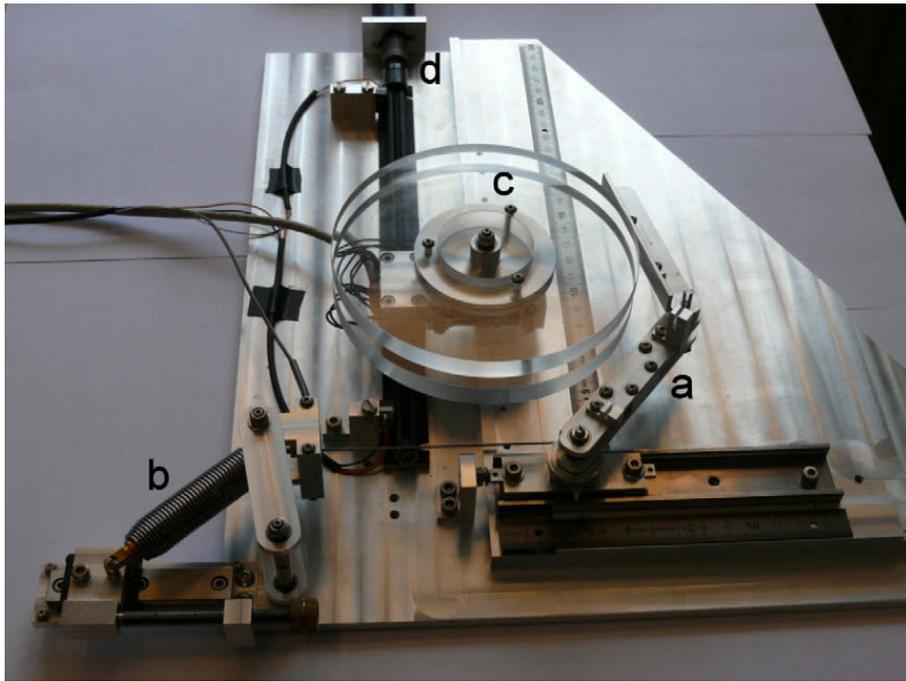
**Fig. 4.** Test set up with underactuated finger (a), constant force actuator (b), cylindrical object (c) and linear motor (d) in order to pull the object out of the hand at a constant velocity.
