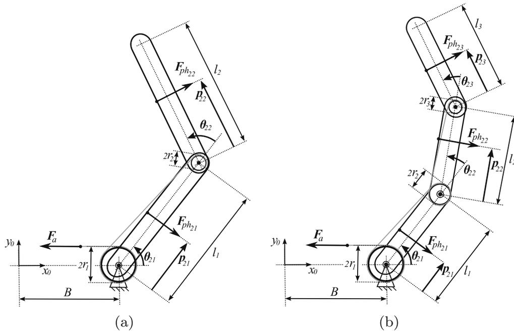
**Fig. 3.** Schematic illustration of the right finger consisting of two phalanges (a) and three phalanges (b), respectively. Both types of fingers are driven by one cable which is subsequently wrapped around freely rotating pulley(s) and attached to the distal pulley which is fixed to the distal phalanx. The radii of the pulleys  $r_j$ , the length  $l_j$  of the phalanges, and the magnitude of the constant actuation force  $F_a$  are given in Table 2.
