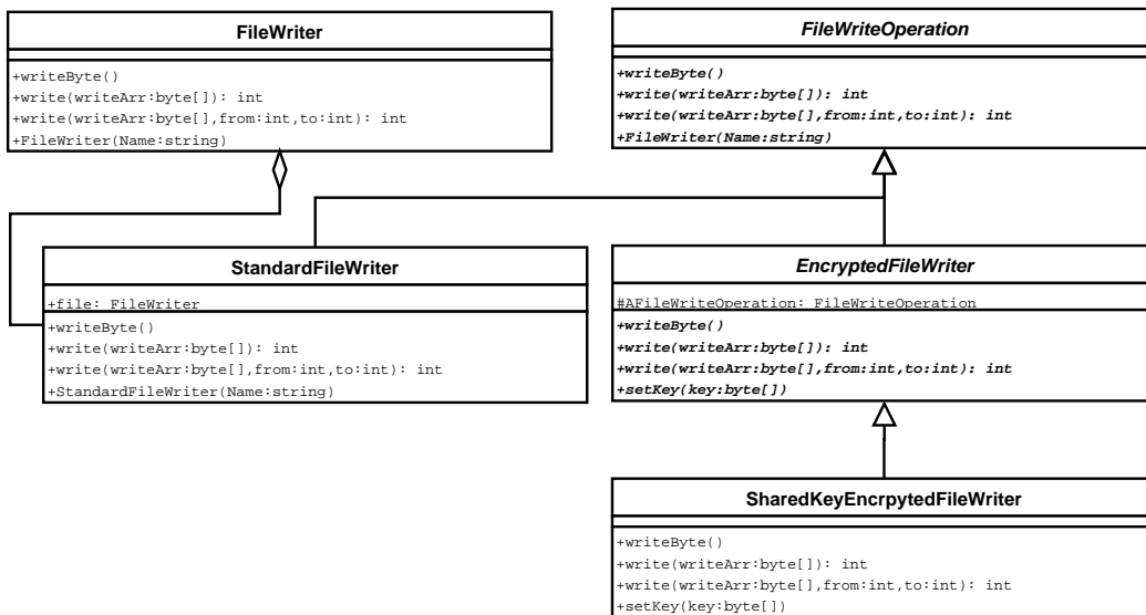
Fig. 3. The system after the addition shared key encrypted file operation using the decorator pattern.
