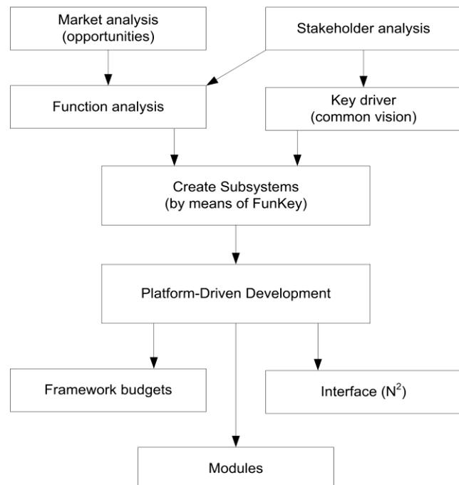
**Figure 5: System design process in the cleaning robot project.**
