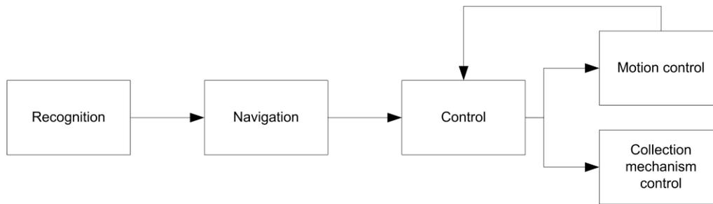
**Figure 4: Basic operation architecture of the cleaning robot.**
