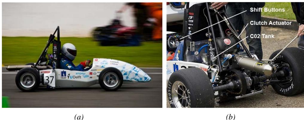
**Figure 5:** One of the DUT Formula Student Cars (a) and its shifting system (b) [Pictures by Jorrit Lousberg].
