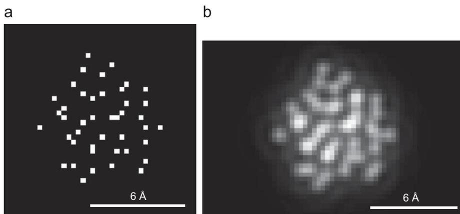
**Fig. 2.** The amorphous Si particle and one of its projections. (a) Top view of the object  $f$ , a Si particle, at the same angle as in Fig. 2b. (b) The noiseless projection  $P$  obtained by multiplying  $f$  with the weights  $W$  for an angle of  $2^\circ$ .
