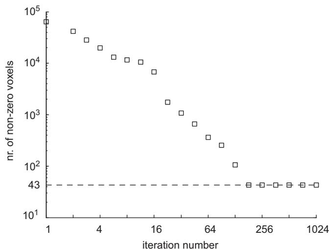
**Fig. 5.** Number of non-zero voxels vs. the iteration number, on a log–log scale. In iteration 181 the mask size reaches the number of non-zero voxels in  $f$ , all atoms are now found. It takes up till the 512th iteration for all the grey values to converge.
