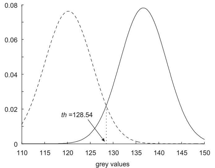
**Fig. 8.** The probability distributions of the value of Al (broken line) and Si (full line). Their respective means are 120.2 and 136.6, the respective standard deviations are 5.2 and 5.1. The threshold  $th$  is put to 128.54.
