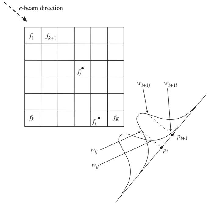
Fig. 1. The atom in position  $j$  gives rise to the right intensity profile, the atom in position  $l$  to the left profile. The resulting image  $p_i$  in  $i$  is the sum of the values in  $i$  of both profiles, i.e.  $p_i = w_{ij}f_j + w_{il}f_l$ .
