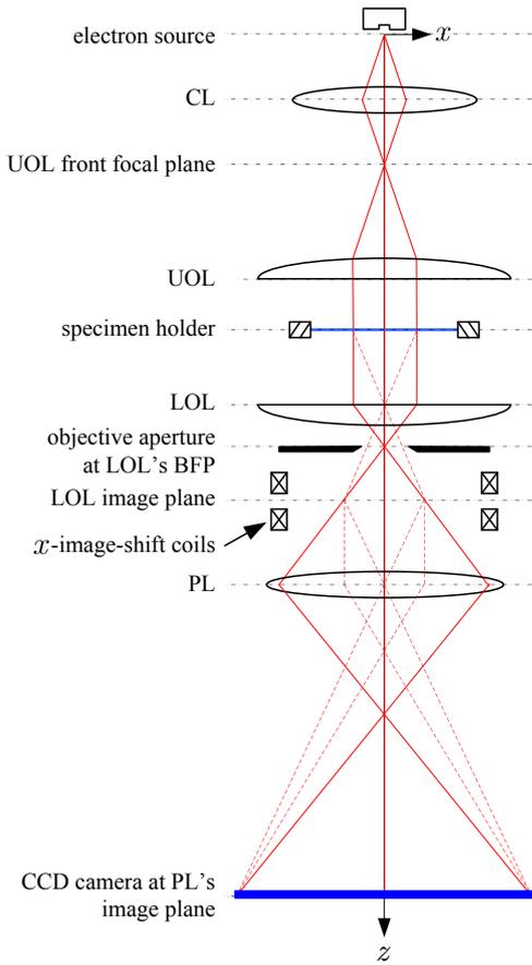
Fig. 1. Main TEM components and amplitude-contrast, bright-field image formation.
