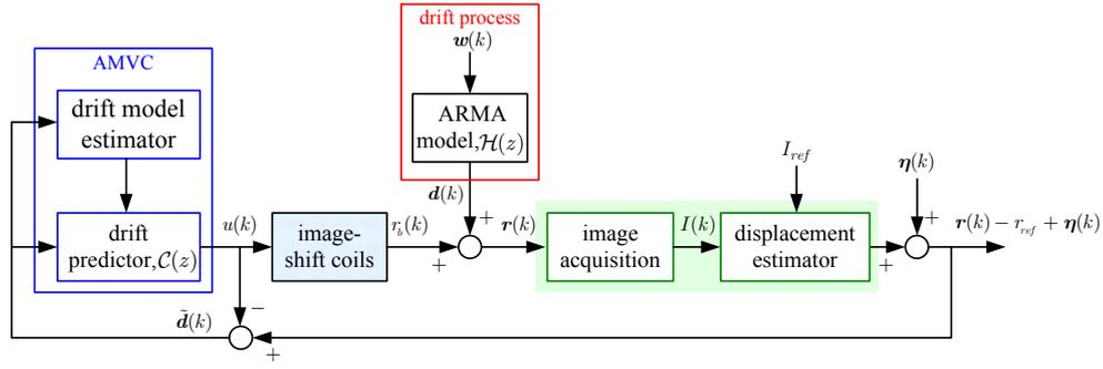
Fig. 2. Main elements of the proposed adaptive minimum variance control scheme for drift compensation.
