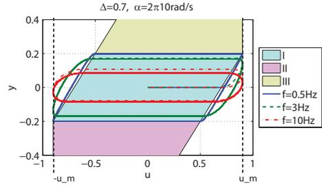
Fig. 5. Convergence of a single section of the nonlinear feedback model to an orbit  $\phi$ . The initial condition is set to 0. In all three cases a sine-wave excitation is used.
