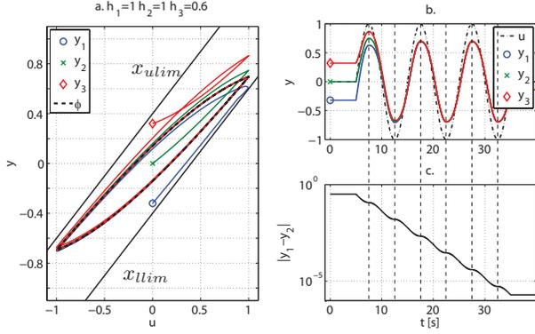
Fig. 1. Simulation of the Duhem model (12) for different initial conditions. a. The input-output plot  $(u, y)$ . The dashed line shows the closed orbit  $\phi(u_T)$ . b. The response for  $u_T = \sin(2\pi/T)$ ,  $T = 10$  s in the time-domain. c. The difference between trajectories  $|y_1(t) - y_2(t)|$  on a logarithmic scale.
