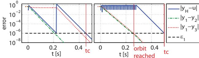
Fig. 7. Difference between the trajectories on a logarithmic scale.  $|y_1 - y_2|$  vanishes for  $u = u_m$ ,  $|y_1 - y_3|$  for  $u = -u_m$ . (Compare with Fig. 6.). The error signal  $|y_H - u|$  denotes the linearized case, which provides the initialization time.  $\epsilon_1$  denotes the allowed error.
