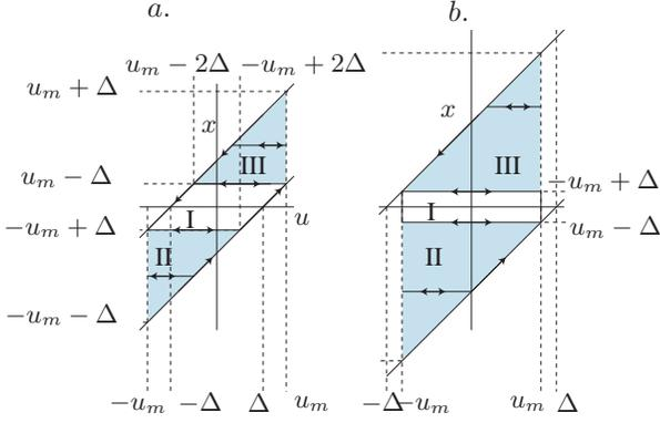
Fig. 3. Illustration of two play operators *a.*  $u_m \geq \Delta$ , *b.*  $u_m < \Delta$
