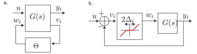
Fig. 4. Block diagram of a nonlinear feedback model. Left *a.* the general version with static nonlinearity  $\Theta$ . Right *b.* The specific implementation with dead-zone analyzed in this paper.
