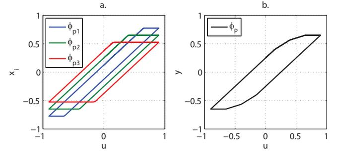
Fig. 2. Illustration of the multi-play hysteresis model(15) with  $\Delta_1 = 0.25, \Delta_2 = 0.5, \Delta_3 = 0.75$ ,  $w_{1,2,3} = 1$ ,  $x_{01} = x_{02} = x_{03} = 0$ ,  $u_T = 0.9 \sin(\pi t)$ .
