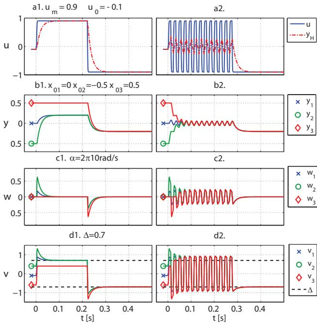
Fig. 6. Simulation of the nonlinear feedback model for three initial conditions with equal  $\Delta$  and equal  $\alpha$ . Begin and end conditions are  $u_0$  and  $u_e$ . All intermediate signals  $y, w, v$  are shown. Subplot a. shows the response of the linear case  $y_H$  where  $\Delta = 0$ .
