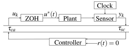
Fig. 1. Schematic overview of the networked control system.
