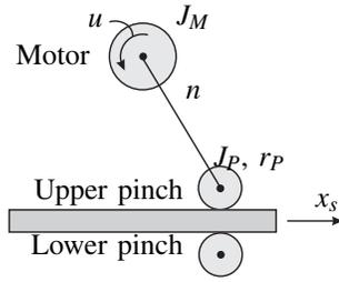
Fig. 2. Schematic overview of the motor-pinch example
