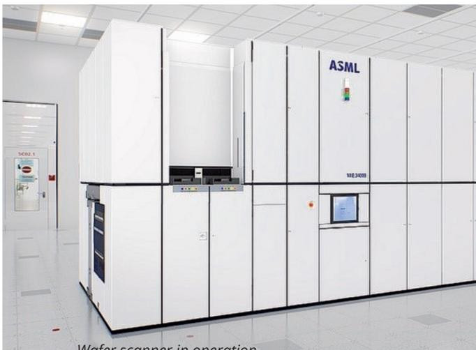
Wafer scanner in operation
