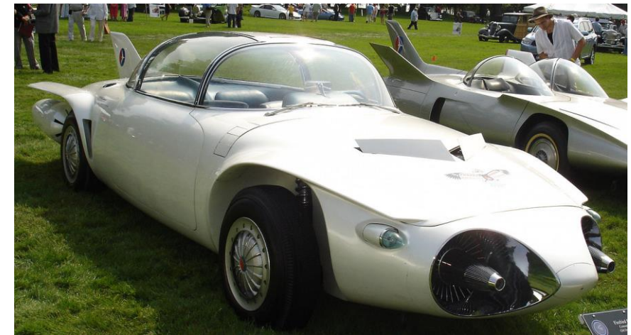
GM Firebird II having an "electronic brain" that allowed it to follow a lane
